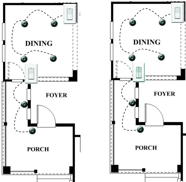
If you want to be able to control the porch and dining room lights separately, but also want to control BOTH circuits from BOTH switch locations, replace the double rocker near the porch door with a triple rocker and replace the single rocker near the entry to the dining room with a double rocker.
